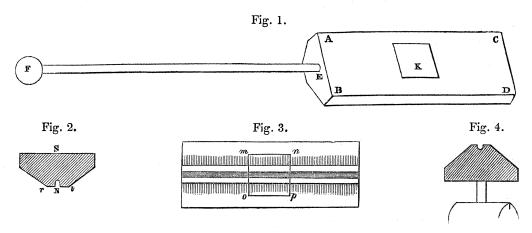
of the rocker, showing the groove underneath; the depth SN is 0.5 of an inch.
